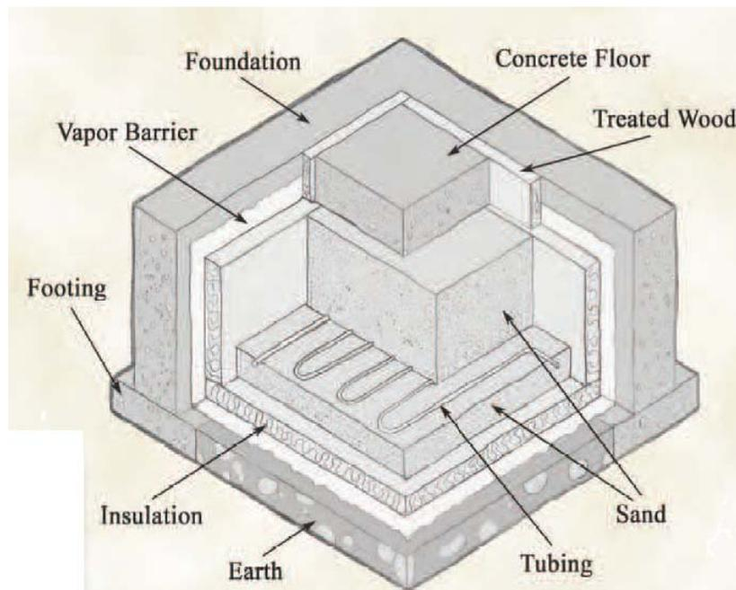
**Figure 1.** Schematic of the sandbox underneath the home used for seasonal storage [Ramlow, 2008].
