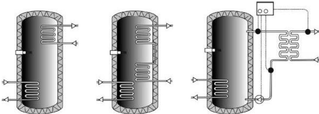
**Figure 4.** The tank to the far left shows a single internal heat exchanger that can retrieve about 40% of the input thermal energy. The middle tank has two internal heat exchangers and can retrieve about 70% of the input thermal energy. The tank on the right is an external heat exchanger and can retrieve up to 80% of the input thermal energy [Nielsen, 2006].
