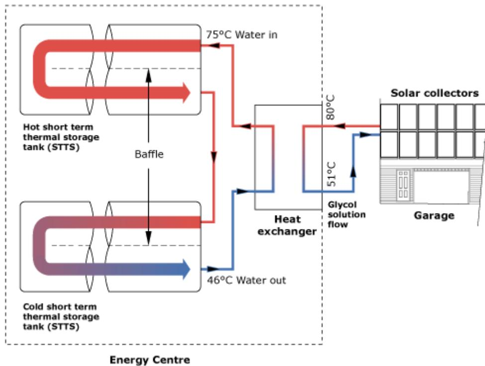
**Figure 3.** Schematic of the Energy Centre heat exchanger at Drake Landing [Drake Landing, 2009].
