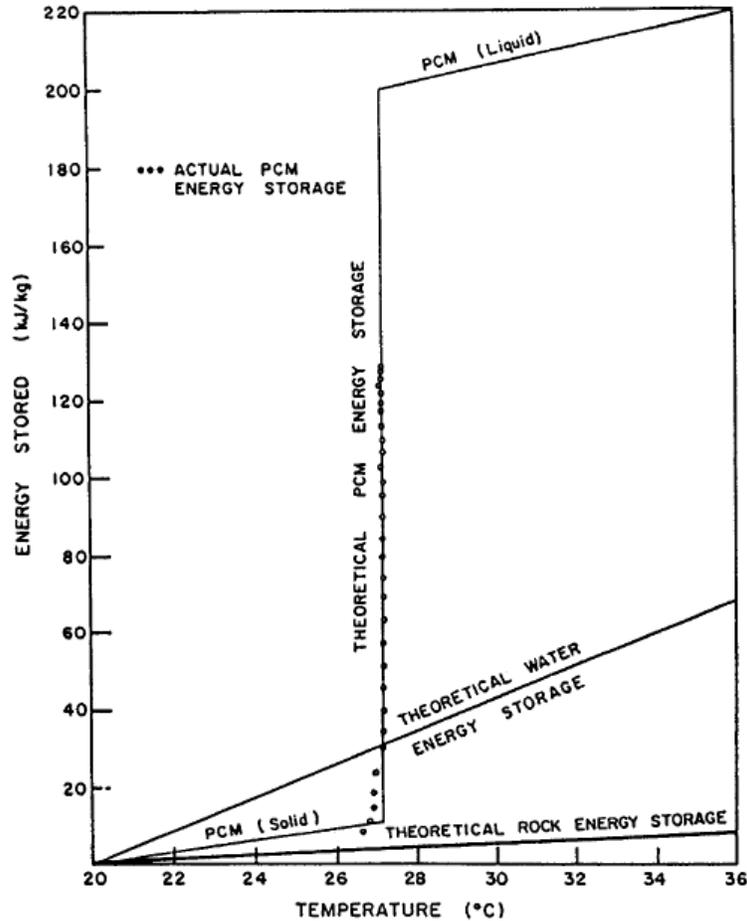
**Figure 9.** Performance comparison of a PCM to sensible heat storage [Kaygusuz, 1999].
