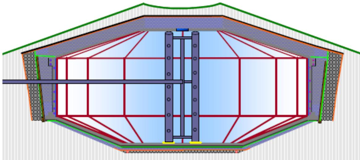
**Figure 5.** Underground water tank constructed in Munich, Germany. The upper image shows the construction layout while the bottom image shows the center stratification device [Schmidt, 2006].
