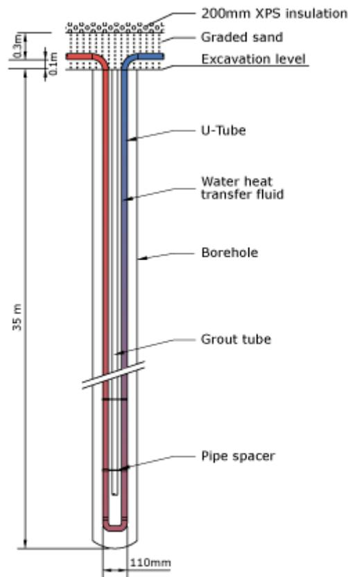
**Figure 6.** A closed loop borehole used at Drake Landing [Drake Landing, 2009].
