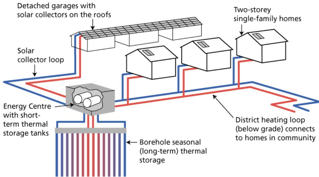
**Figure 2.** Schematic of Drake Landing showing the detached garages with solar collectors, the energy center, borehole storage, and district heating loop [Drake Landing, 2009].
