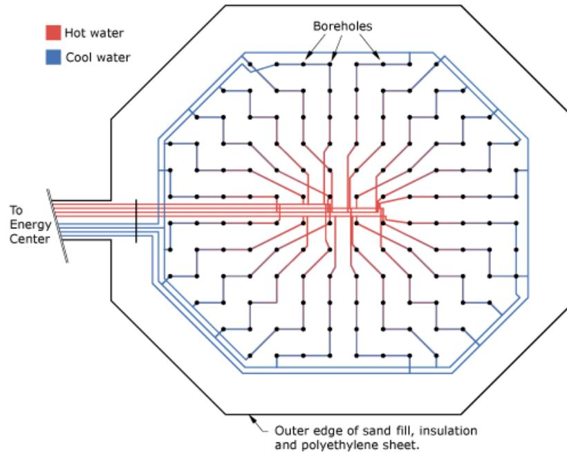
**Figure 8.** Schematic of the warm working fluid starting at the center and moving outward of Drake Landing. There are 24 parallel sets of 6 boreholes in series (144 boreholes) beginning and ending at the Energy Center heat exchanger [Drake Landing].
