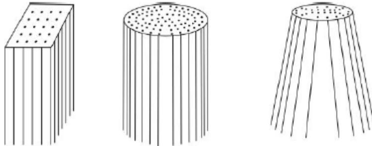
*Figure 7. Examples of different borehole drilling patterns commonly used [Nielsen,2006].*
